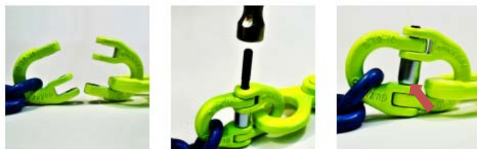
Fig. 4 Gunnebo instructions of assembly with clamping sleeve upside down (red arrow)
