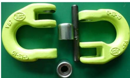
Left: Gunnebo G-coupler (or 2 x SKT) with clamping sleeve and SKA bolt. Fittings varnished in dark yellow are usually grade 8 steel, light yellow indicates grade 10. Pins are only available in grade 10 steel.
