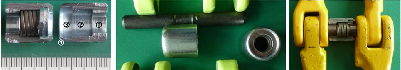
Left: Buildup of sleeve with drilled hole for pin ① spring ② and washer ③, curved edge (flattened rim) of the sleeve ④.
