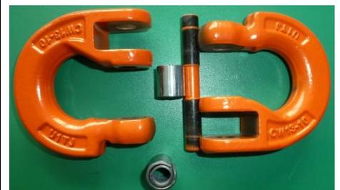
In the case of the PEWAG CBHW model (components of similar manufacturing are also made by other producers), the pin is secured by an inner and an outer clamping sleeve. The inner sleeve clasps the notch of the pin and the outer sleeve provides secure fastening.
