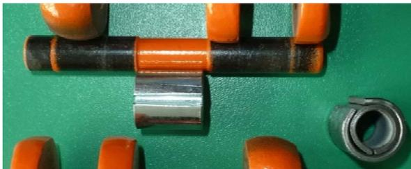
The sleeve consists of 2 clamps made of spring steel. Compared to the Gunnebo model, a striking feature is the identical width of notch and sleeve.
