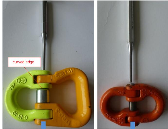
Driving out of the pin with the help of a pin punch of proper size (Ø slightly smaller than sleeve's). Use a solid support with an aperture in the middle: aperture depth = pin length + 5 mm. Gunnebo: the sleeve's curved edge must be ABOVE.
