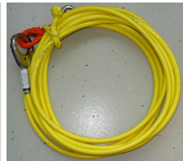
If you wish, tie the flaked rope with a ribbon, shackle or, as in the picture, secure with a textile shackle.
