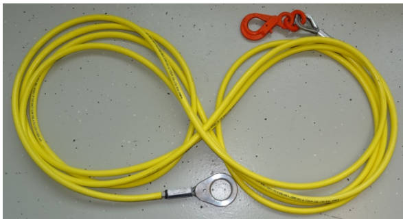
For manual flaking of ropes, see AWA part 1. Picture: rope coiled in a figure eight flake to allow unrestricted deposit.
