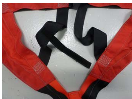
Fig. 3: Reinforcement strap sewn onto left bottom belt
