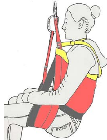
Fig. 6: 10 cm lengthening of crotch strap with a karabiner = slightly more upright sitting position
