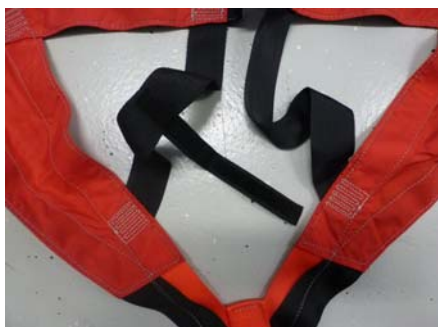
Fig. 3: Reinforcement strap sewn onto left bottom belt
